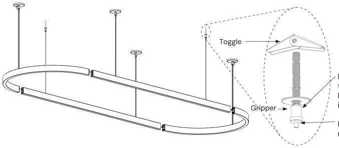
Feed aircraft cable through gripper and exit hole on top. Screw gripper into toggle.
