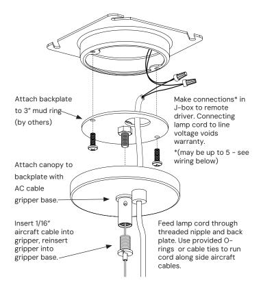
Remote driver housing has options for bar hangers for mount above suspended ceilings. Drivers must remain accessible after finished installation. Multiple driver housings must be spaced minimun 4 inches apart.
