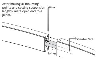
CAUTION: Insert joiner into center slot only. Inserting the joiner into upper or lower LED slots will result in damaged and/or broken LEDS.
